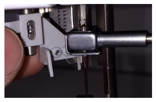
Tighten the screw up just enough to allow you to move the threader up and down slightly on the shaft and then line up the threader hook so that the threader hook is at the top of the needle eye. Then tighten the screw.
