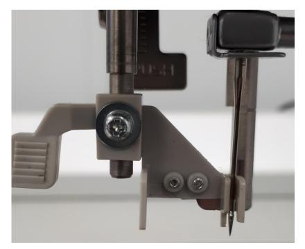
To fit the needle threader, you will need to slide the threader over the shaft and line up the screw with the hole in the shaft.
