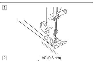
1 Loosen the thread tension to "1" and increase the stitch length to 5.0.
