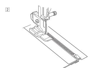
2 Attach the zipper foot E with the pin on the right hand
