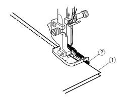
Attach 1/4" seam foot O, which helps you to keep a constant 1/4" (6 mm) seam allowance.
