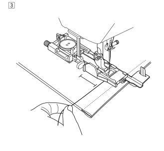
3 Place the fabric between the buttonhole foot and stabilizer plate. Lower the needle into the starting point by turning the hand wheel.
