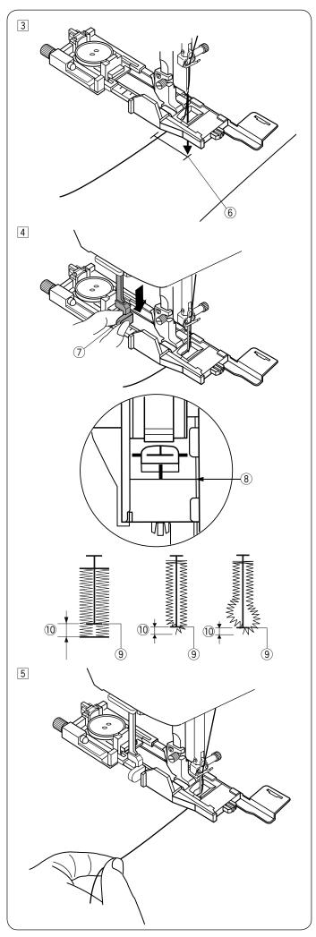
3 Draw the needle thread to the left through the hole of the foot.
