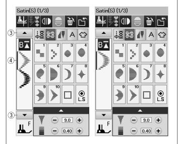
To delete a pattern in the middle of a combination, press the cursor key to select the pattern you wish to delete. The stitch image of the selected pattern turns blue. Press the delete key to delete the selected pattern.
