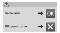
When you stop the machine, a message will appear. Press the OK key and the machine memorizes the seam length to sew another piece of the same length. Press the X key to sew in a different size.
